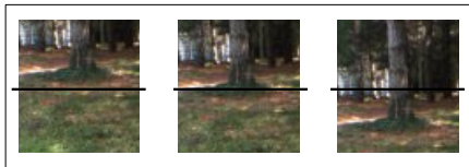
Fig. 2. The 3 possible labels: left : the foot line is on open ground, so label = ground; center : the base of the object is on the foot line, so label = obstacle; right : the foot line is blocked by a nearby object, so label = blocked.
