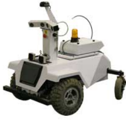
Fig. 1. The LAGR platform is a non-holonomic (differential drive) off-road mobile robot measuring 1.2m of length by 0.74m of width by 1.02m of height. It weighs 109kg and can travel at up to 1.3 meters/seconds. Despite its relatively small size, such a vehicle presents dynamics that cannot be ignored in a collision-free autonomous navigation system.
