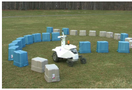
Fig. 9. Comparison of old steering-angle system (red) versus new learned-trajectories system (green). Both systems were run 1 to 3 times over 5 different 30 meter courses each consisting of a different arrangement of buckets as obstacles with gradually increasing difficulty (left: slalom course). Running times and number of obstacle hits are reported. The hardest course could not be completed by the steering-angle system because the course was systematically destroyed by obstacle hits.
