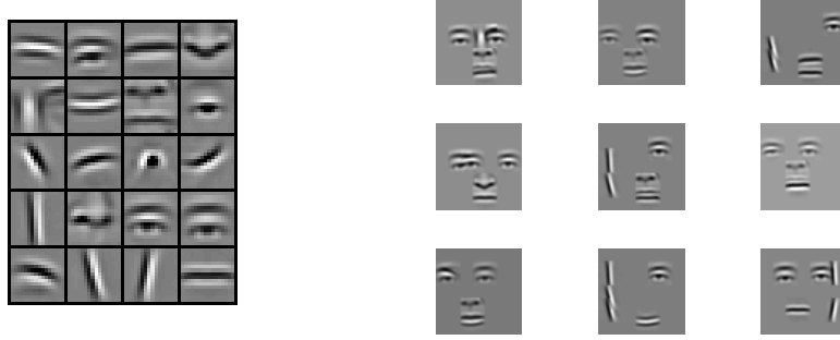
Figure 5: On the left: the dictionary of 16 \times 16 filters learned by the convolutional model on faces. On the right: some low energy configurations, generated randomly as in Section 3.5 . Each active filter has response 1.
