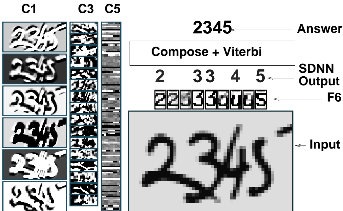
Figure 6: An example of multiple character recognition with SDNN. With SDNN, no explicit segmentation is performed.
