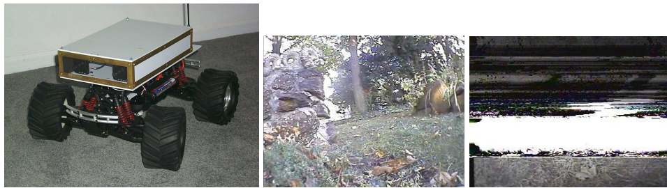
Figure 1: Left: The robot is a modified 50 cm-long truck platform controlled by a remote computer. Middle: sample images from the training data. Right: poor reception occasionally caused bad quality images.
