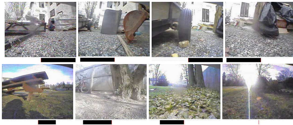
Figure 4: Snapshots from the left camera while the robots drives itself through various environment. The black bar beneath each image indicates the steering angle produced by the system. Top row: four successive snapshots showing the robot navigating through a narrow passageway between a trailer, a backhoe, and some construction material. Bottom row, left: narrow obstacles such as table legs and poles (left), and solid obstacles such as fences (center-left) are easily detected and avoided. Highly textured objects on the ground do not detract the system from the correct response (center-right). One scenario where the vehicle occasionally made wrong decisions is when the sun is in the field of view: the system seems to systematically drive towards the sun, whenever the sun is low on the horizon (right). Videos of these sequences are available at http://www.cs.nyu.edu/~yann/research/dave/index.html .
